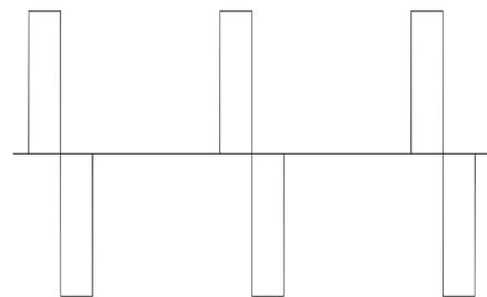
Figure 9.4—Biphasic Waveform
