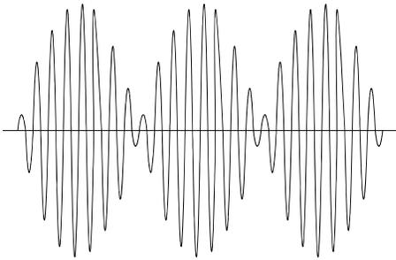
Figure 2—Premodulated Waveform
