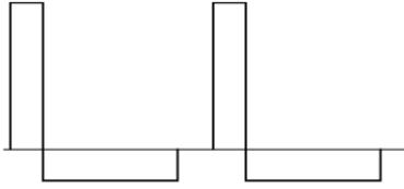
Figure 8—TENS Asym. Waveform
