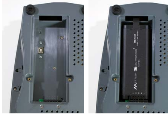
Figure 3.2— Sys*Stim 240, Bottom View— Installing the battery
