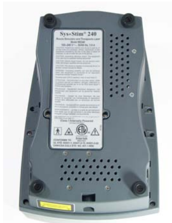
Figure 3.1— Sys*Stim 240, Bottom View Showing battery door
