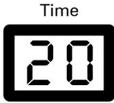
Time display shows time remaining in treatment in whole minutes. When the unit is first turned on the time display will show 15 minutes. You can set any time from 1-60 minutes.
