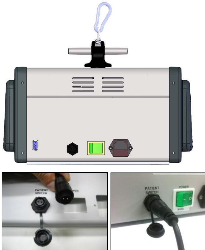
Figure 5.2— Rear View of the MTD 4000 Showing Connectors and Switches
